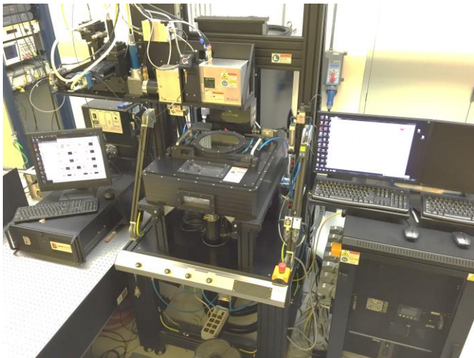
Open architecture Fraunhofer 3D printer
