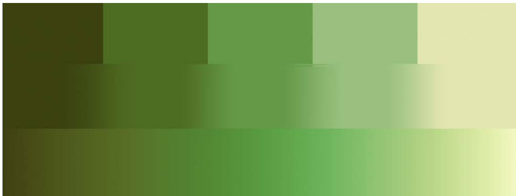
Figure 22: Construction of a green colorscale that moves from a warm dark yellow-green through a mid-range cool blue-green and back to a warm light yellow-green. This allows the colorscale to maintain intuitive order while moving between warm and cool greens – shifts that create additional contrast.
