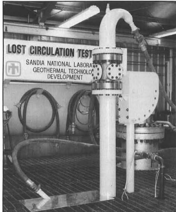
Figure 4 We designed this lost-circulation test facility to resemble the Halliburton facility in Duncan, Oklahoma. The equipment realistically simulates flow of non-Newtonian drilling muds, cements, and lost-circulation materials from
