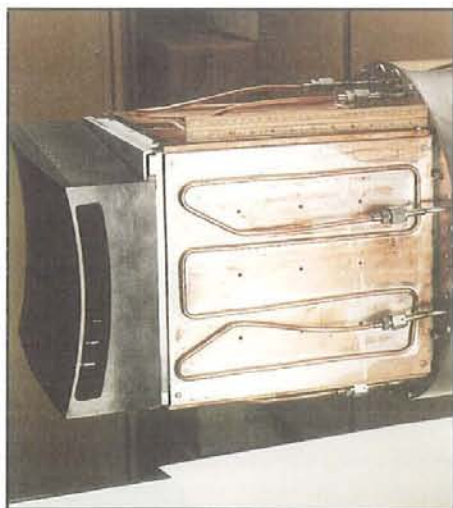
Figure 5 View of ALT-I module showing instrumentation probes in the throat region.
