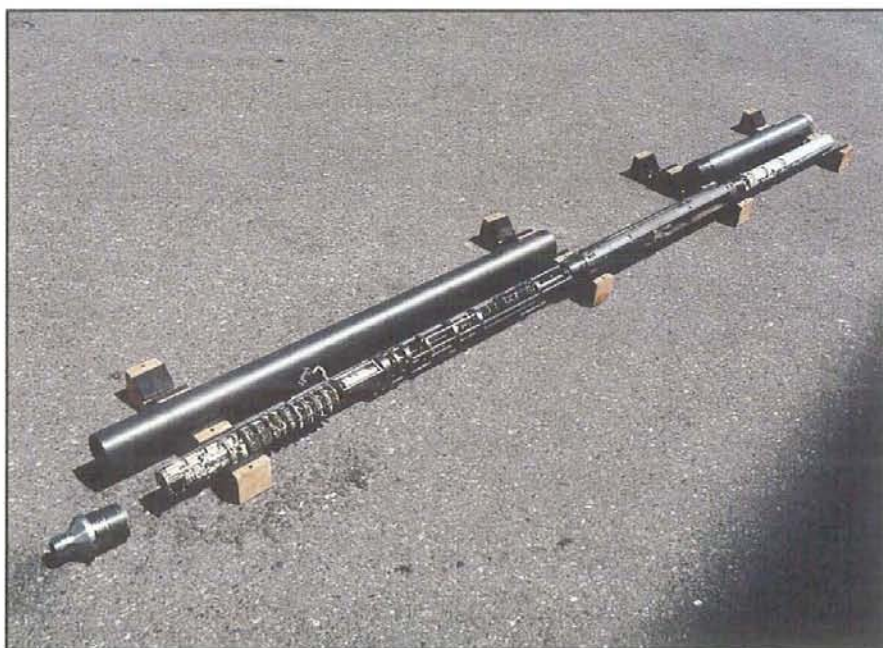
Figure 18 The state-of-the-art borehole seismic tool designed and fabricated by Sandia may play an important role in monitoring energy extraction processes ranging from thermal to hydraulic stimulation of oil and gas wells.
