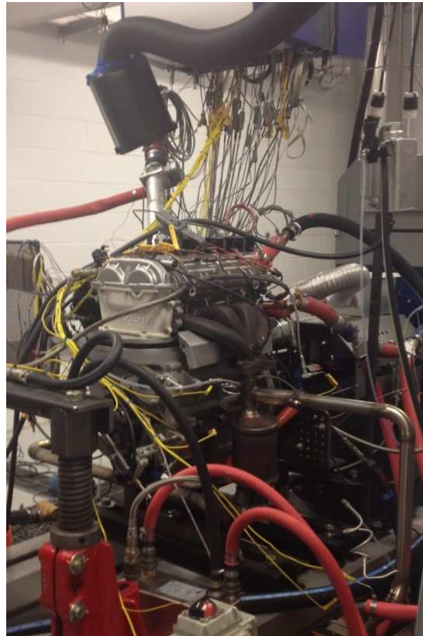
Figure 15. Envera VCR engine at MAHLE Powertrain.
