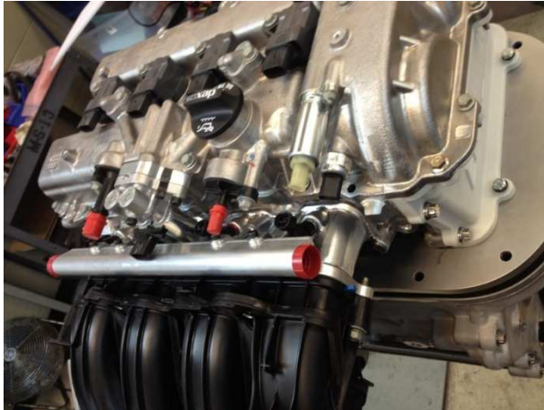
Figure 16. PFI fuel rail added to the stock GDI cylinder head.
