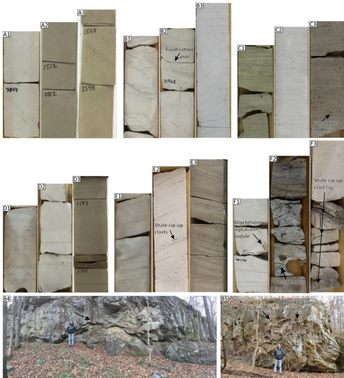
Figure 3.4. A) Lithofacies SM. Left to right: (A1) 930.9 m (3054 ft) RHF #2-S (API 120650139400); (A2) possible distorted bedding, 471.8 m (1548 ft), Heckert #902 (API 120512572400); (A3) 460.9 m (1512 ft), Heckert #902. B) Lithofacies D. Left to right: (B1) 903.1 m (2963 ft), RHF #5-S (API 120650139200); (B2) 902.8 m (2962 ft), RHF #2-S (API 120650139400); (B3) 32.6 m (107 ft), Tripp #1; (B4) 469.4 m (1540 ft), Heckert #902; (B5) Domal structure from north Cypress Creek, (B6) Large-scale fluid escape structure from north Cypress Creek. C) Lithofacies SR. Left to right: (C1) 865.9 m (2841 ft), RHF #4-S (API 120650135600); (C2) poorly developed asymmetric ripples 29.6 m (97 ft), Tripp #1; (C3) oil stained and iron oxide, 881.5 m (2892 ft), Coen #120 (API 121592608300); D) Lithofacies SP. Left to right: (D1) 901.0 m (2956 ft), RHF #5-S; (D2) 901.9 m (2959 ft), RHF #2-S, (D3) low angle, 470.3 m (1543 ft), Heckert #902. E) Lithofacies SC. Left to right: (E1) non-oil stained 881.2 m (2891 ft), RHF #5-S, (E2) shale rip-up clasts on foresets 42.1 m (138 ft), Tripp #1, (E3) oil-stained 790.7 m (2594 ft), Montgomery #B-34 (API 121592606400); F) Lithofacies C. Left to right: (F1) shale rip-up clast and rounded septarian nodule lag from within thick Western Belt Sandstone 922.3 m (3026 ft), RHF #2-S, (F2) calcareous fossiliferous lag from within thick Western Belt Sandstone 891.5 m (2925 ft), RHF #5-S, (F3) shale rip-up clast lag at the base of thick Western Belt sandstone 56.7 m (186 ft), Tripp #1.
