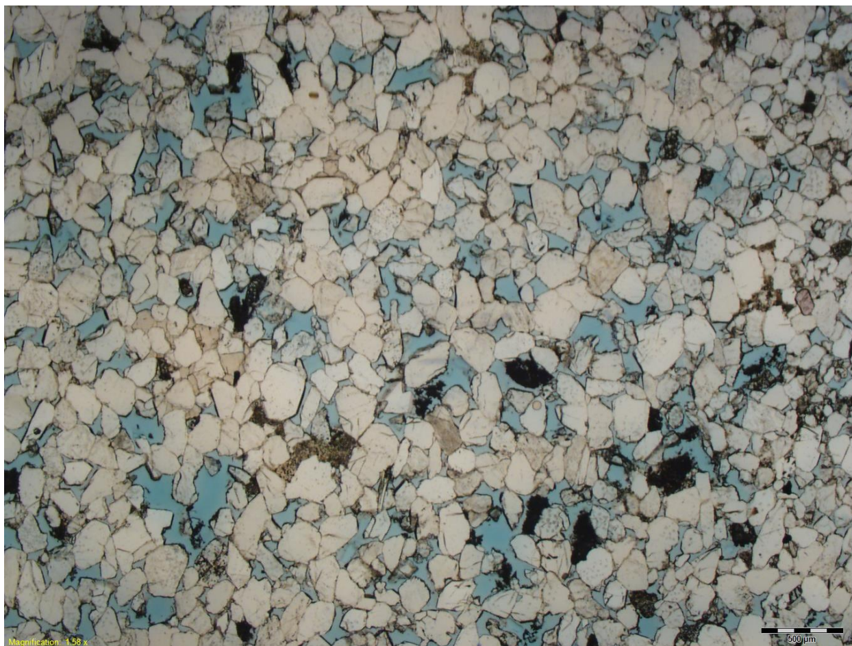
Figure 3.73. Montgomery #B-34 at 790.2 m (2592.5 ft), S_c , \Phi = 20.1\% , k = 2.56 \mu\text{m}^2 (2592.5mD), 2.5X plane polarized light. The scale bar at bottom right is 500 \mu\text{m} .
