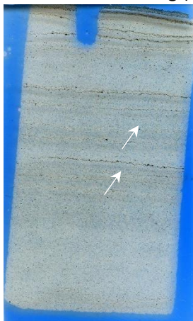
Figure 3.48. Scanned thin section showing fine bedded silt layers (indicated by white arrow) at RHF #2-S (APR 120650139400) 2954.8'.
