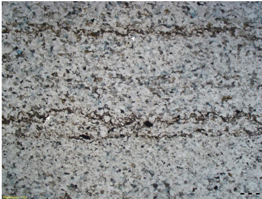
Figure 3.49. Fine bedded silt layers (indicated by white arrow) from the previous thin section under the microscope with 5x objective under plane polarized light, scale bar down right is 200 \mu\text{m} .
