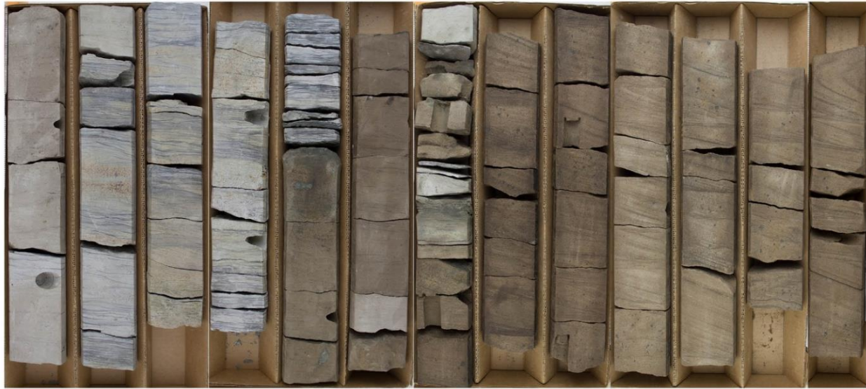
Figure 3.14. The top of the Montgomery #B-34 core is in the upper left corner and proceeds downhole toward the bottom right. Each box segment is 0.6 m (2 ft) long. The core shows a typical upward change in facies from dominantly cross-bedded and ripple-bedded sandstone to heterolithic strata above. The change in color of the core from light brown to light gray reflects the lack of oil staining in the nonreservoir heterolithic facies. Figure 3.15 shows a graphical depiction of facies in the Montgomery core.
