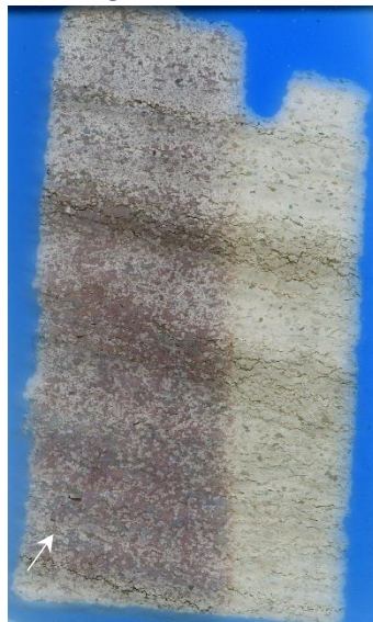
Figure 3.50. Scanned thin section with left side stained with dual-carbonate staining, calcite cement stained with a red color (indicated by white arrow) RHF #2-S (API 120650139400) 3050.4'.
