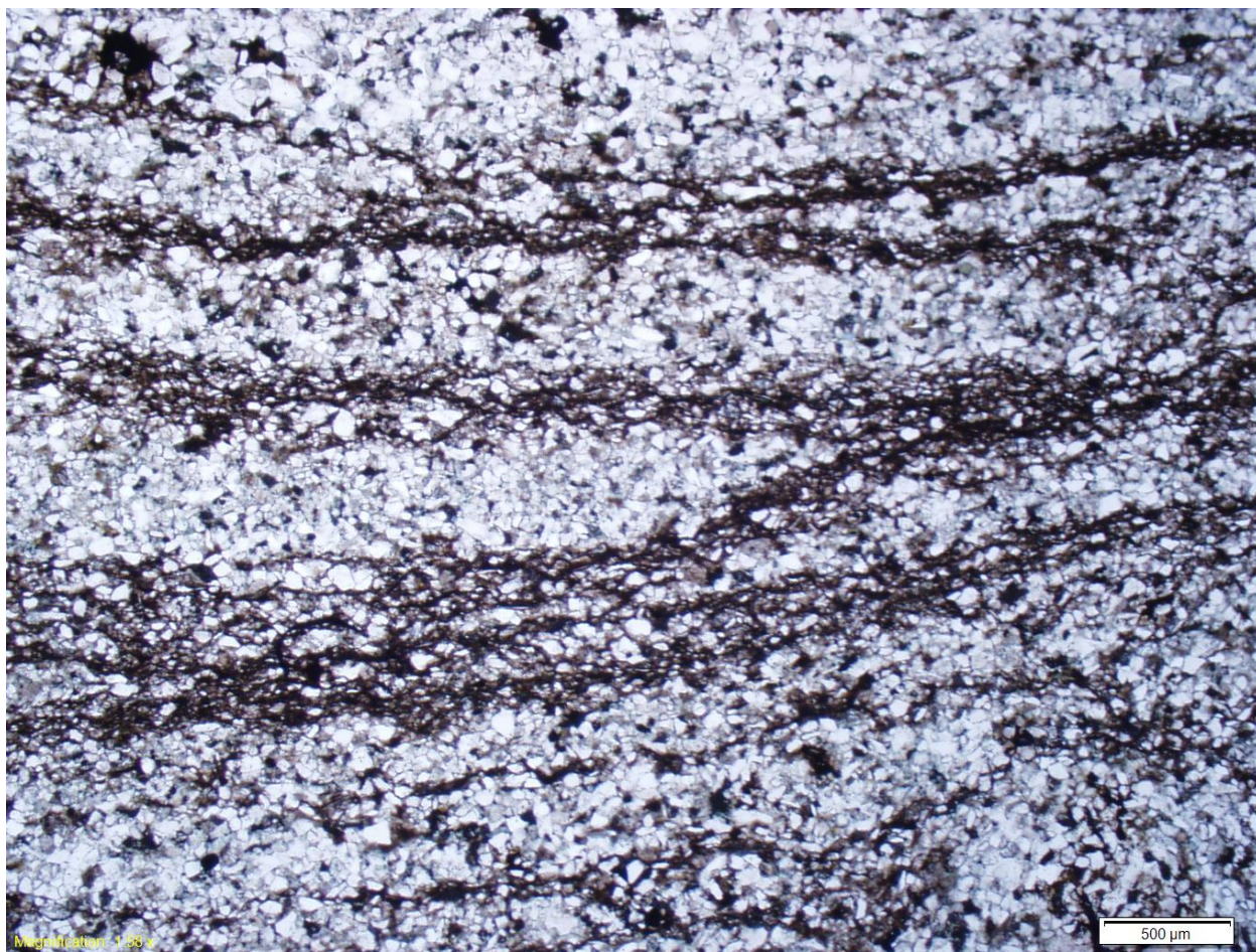
Figure 3.70. SRD facies sandstone thin section, Montgomery B-34, API# 121592606400, at 2583.5'. 2.5X plane polarized light. The scale bar at bottom right is 500 \mu\text{m} .
