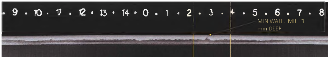
Figure 8. Digital X-Ray of IC Weld
