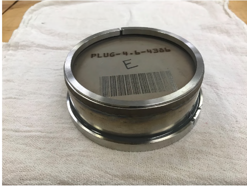
Figure 3. Sample Lid with Attached Seal Ring
