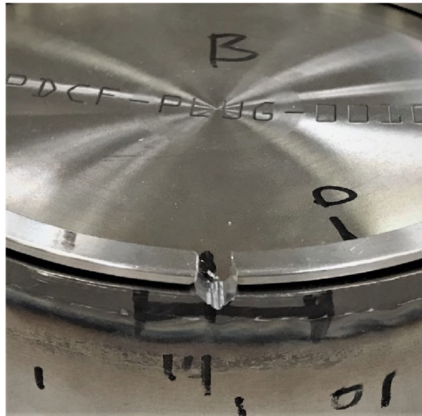
Figure 9. Photo of Machined Leak Location
