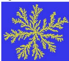
Figure 1. Schematics of the structure of 2D clusters formed by aggregation without relaxation.
