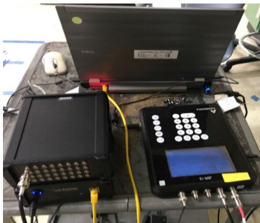
Fig. 4. The electronics for data collection and signal processing are shown with the ALMM (left) and the JSR-15 (right).
