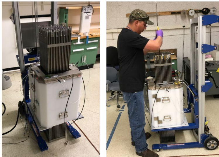
Fig. 3. The complete collar system that surrounds the LANL mockup fuel assembly where hinges for the removable door are shown (right).
