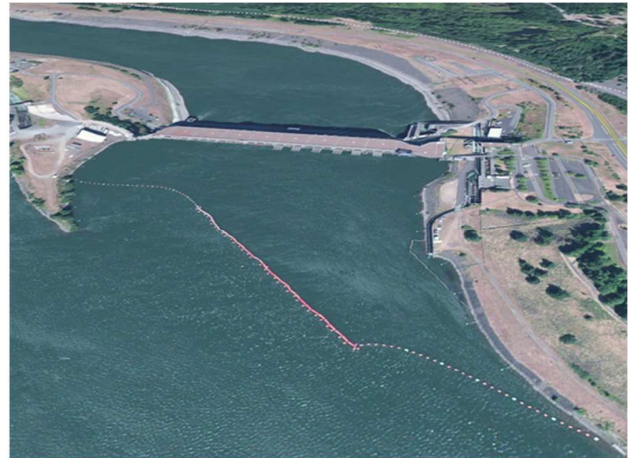
Figure 1: Partial-depth, floating, guide wall. The photo on the left (provided by Shane Scott) shows the panels with the floating boom. The photo on the right (taken from Google Earth) shows an installed guidance device at the Bonneville Dam.
