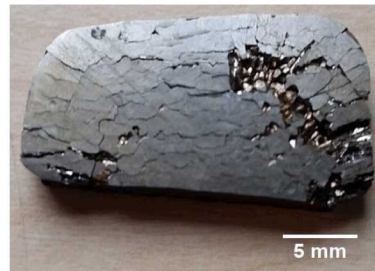
High silicon content electrical steel (Fe-6.5wt%Si)
