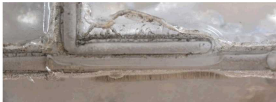
Fig. 4. Post-test image of T-05 block showing region of no detonation.
