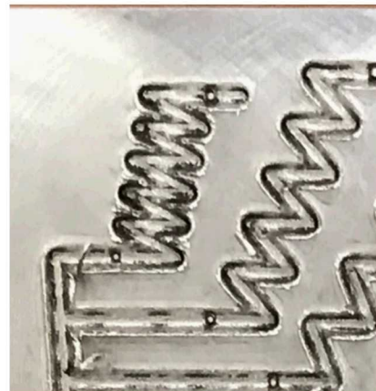
Fig. 11. Results of aluminum switchback test showing detonation in all angles tested.
