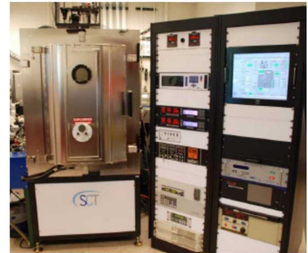
Custom high vacuum chamber for PVD of energetics (top) and schematic of deposition process (bottom).
