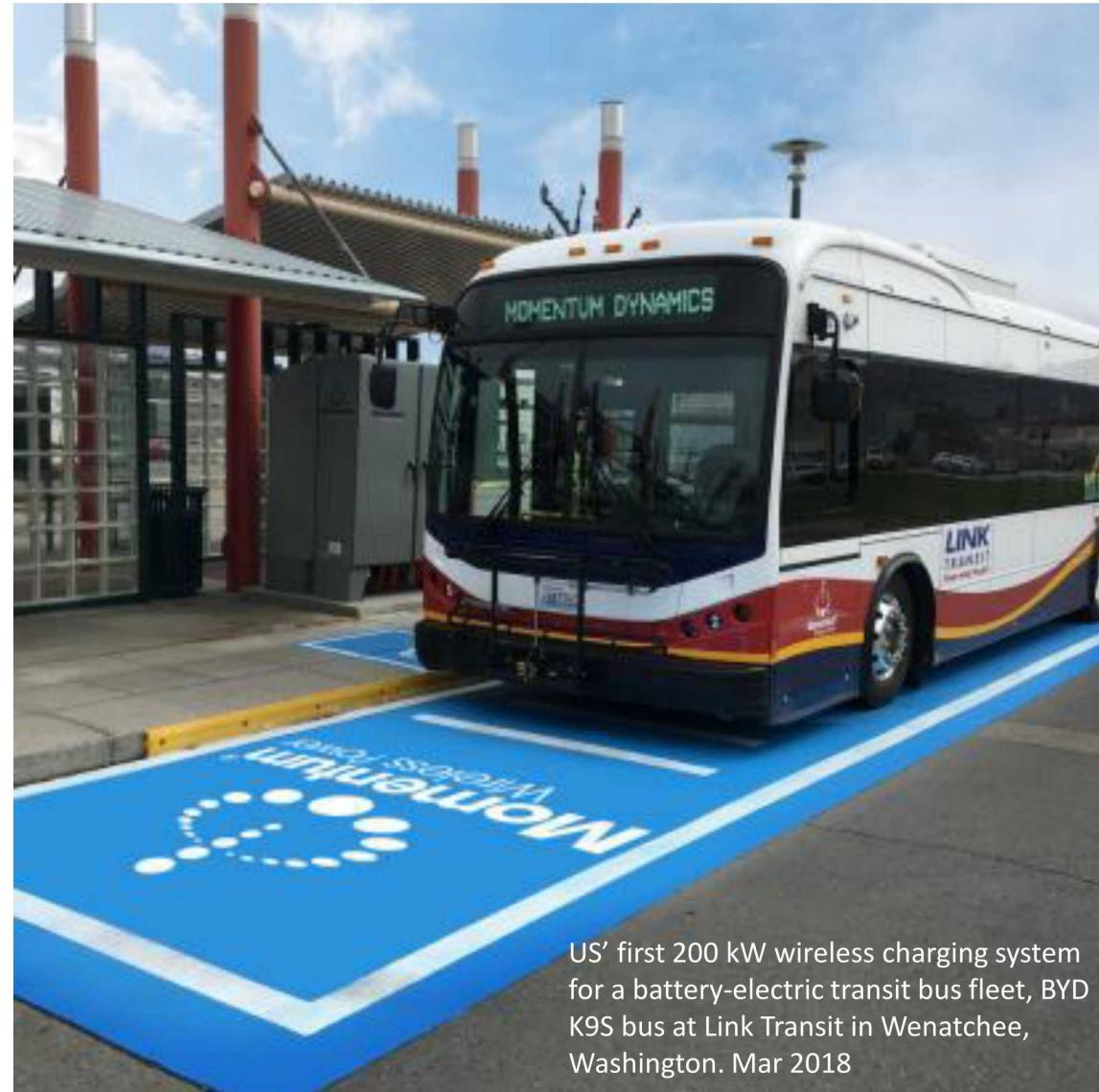
US' first 200 kW wireless charging system for a battery-electric transit bus fleet, BYD K9S bus at Link Transit in Wenatchee, Washington. Mar 2018
