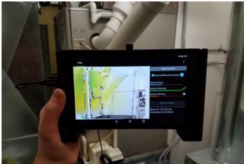
Figure 5. DotProduct structured light sensor. 2
