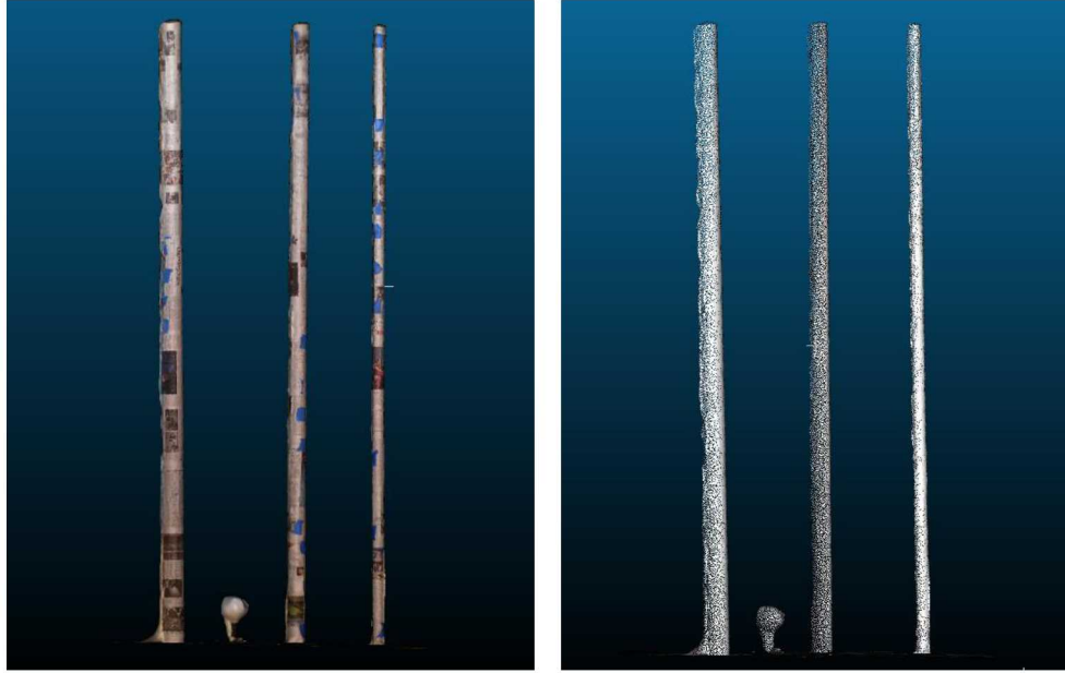
Figure 13. Point cloud obtained by photogrammetry (with artificial texture).
