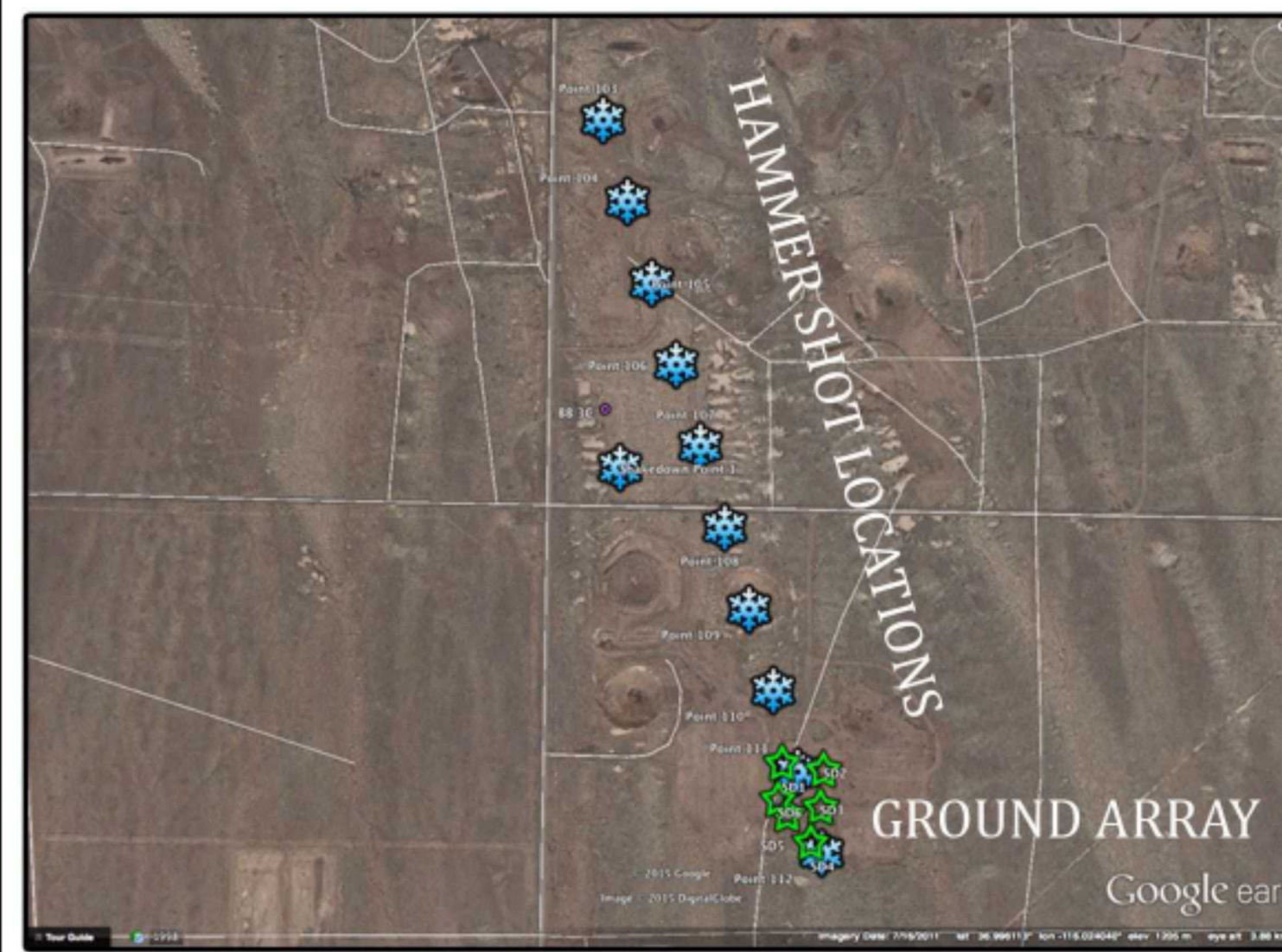
ABOVE: Map showing the 6 Hyperion, seismically decoupled infrasound sensor locations and the hammer shots for the Magni test. The shot point at center left was the "shutdown" shot. The shot series continued from Southeast to Northwest along 200 m increments.
