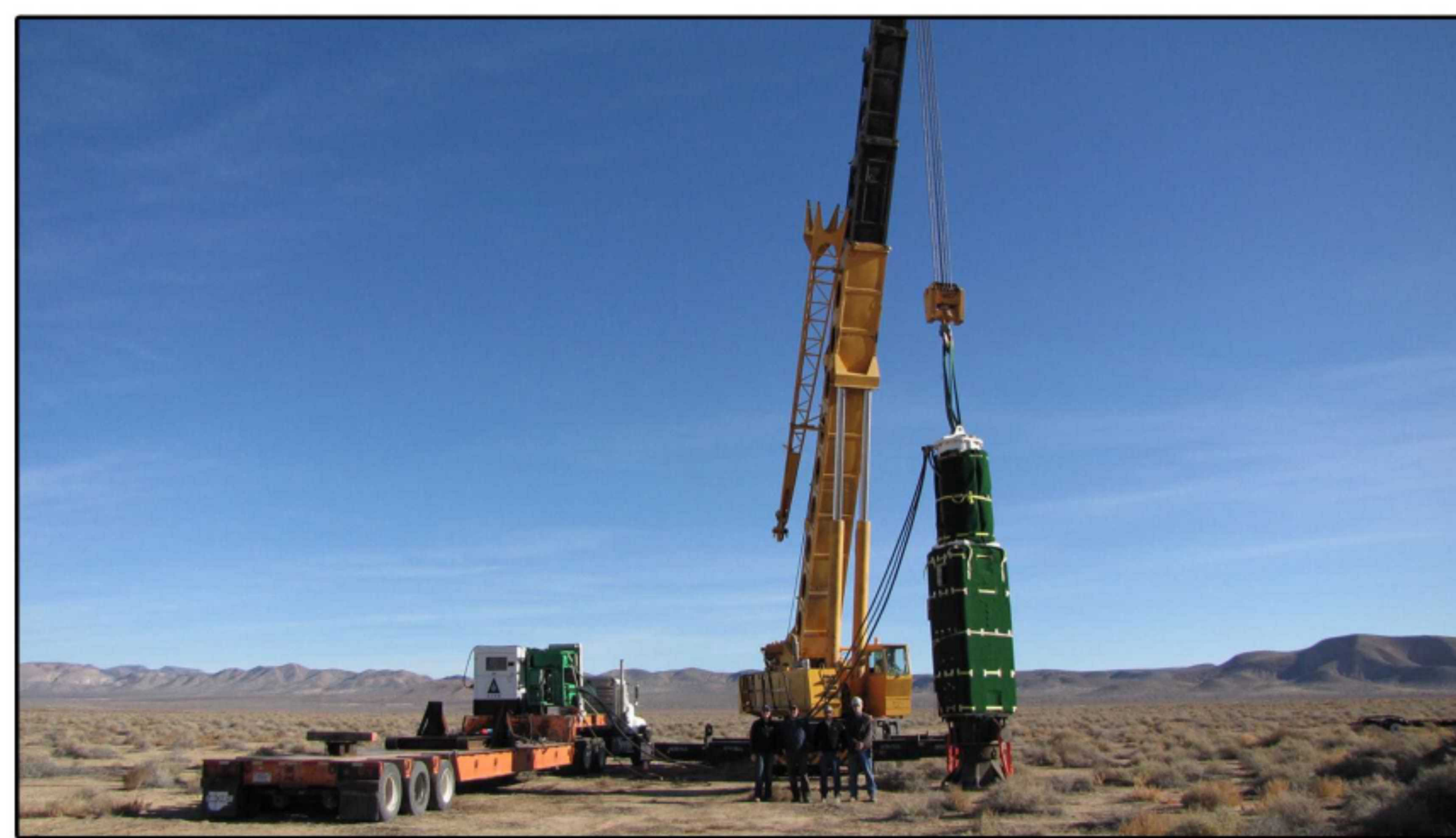
ABOVE: Hammer supported by the crane during the Magni Test. People standing by the hammer for scale.
