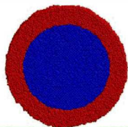
Partially Melted red - liquid 'skin' blue - solid 'core'
