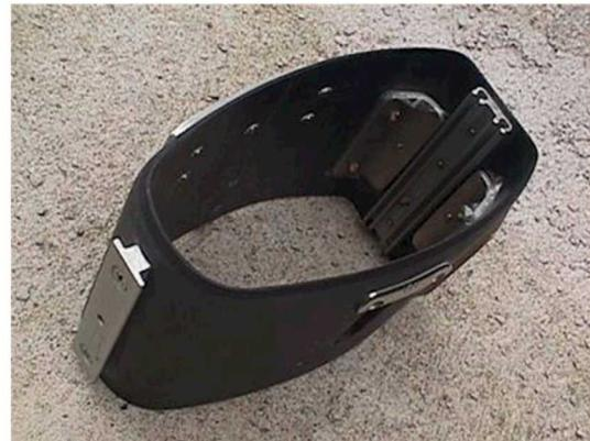
A portion of a carbon fiber composite mast is shown, with metal couplings attached to it. Metal could be Aluminum, steel or other alloy.
