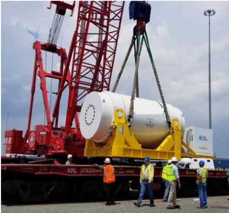
Photo of a mock SNF cask being moved from a container ship to heavy haul truck as part of a multi-modal, multi-jurisdictional international transportation route. Copyright: Sandia National Laboratories.
