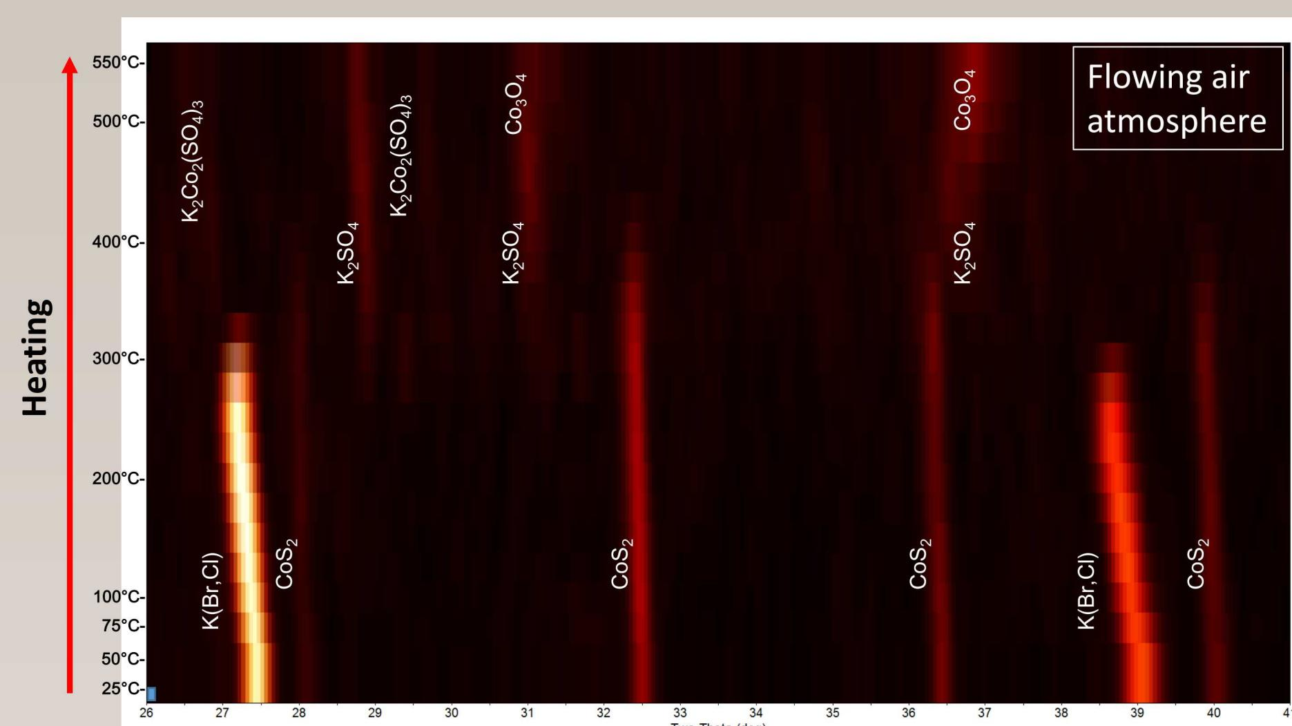
Concurrent Gas Chromatography (GC) measurements made on the gas stream from HTXRD reaction chamber confirmed the release of  $\text{SO}_2$  gas in the 300-450°C temperature range.
