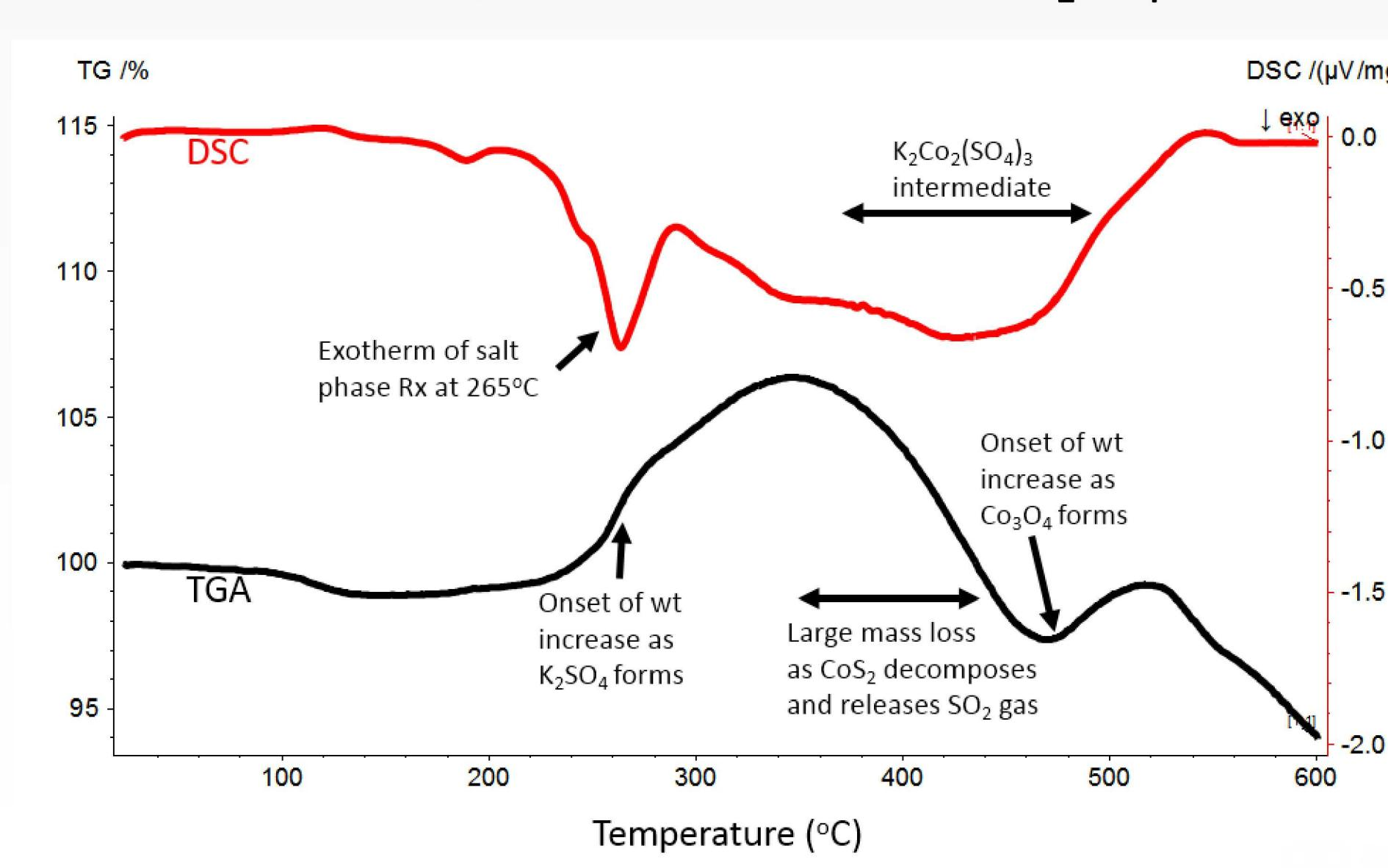
Mass Spectroscopy (MS) results from DSC/TGA analysis confirm  $\text{SO}_2$  gas release with an onset of  $\text{SO}_2$  formation at 265°C when the salt phase starts to react to form  $\text{K}_2\text{SO}_4$ .
