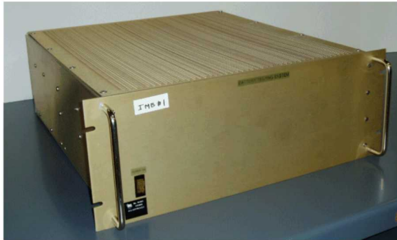
Impedance measurement box developed by INL
