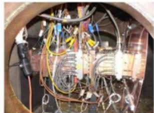
Flow path constructed with 50.8 mm (2 inch) thick copper walls thermally protected with zirconium dioxide coating (144 static pressure ports, 19 flow path surface thermocouples, 4 heat flux gauges)
