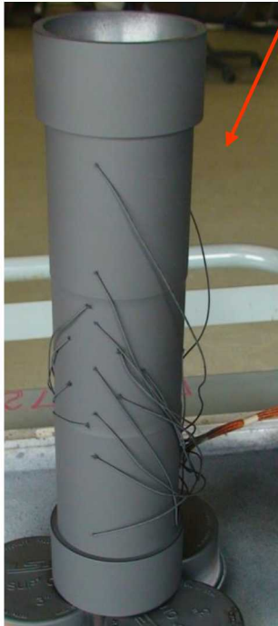
Ceramic slug replaced with stainless steel
