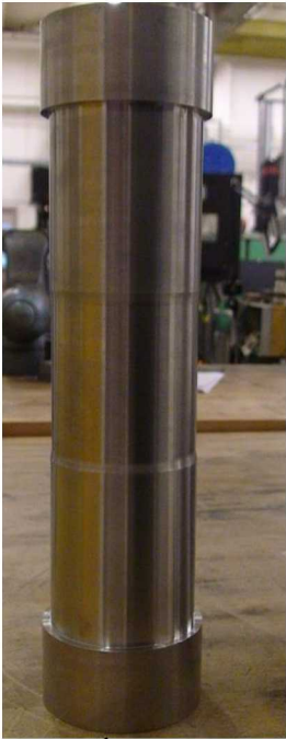
3" Reduced section, from 0.050" to 0.020"
