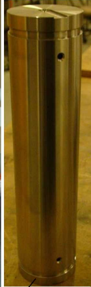
Fixture and specimen geometry modified to allow loading in tension
