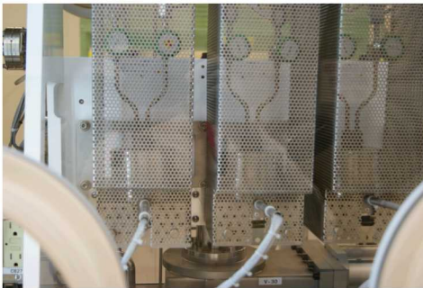
Heat Shields over Heaters
