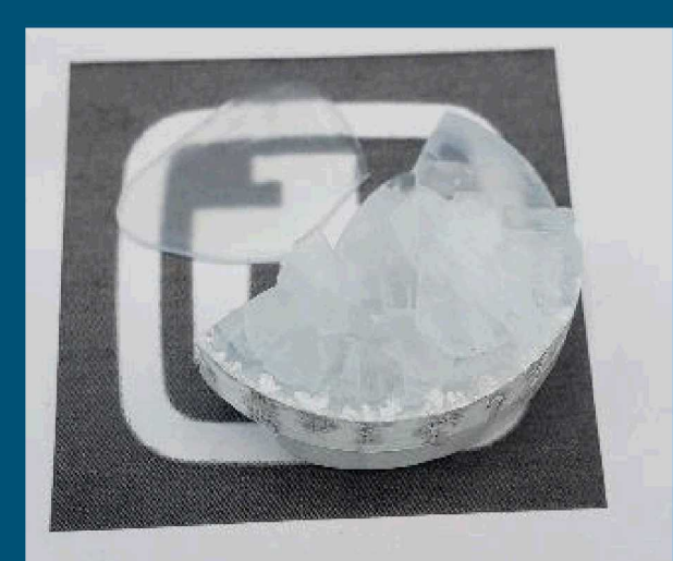
Sub-100°C processing Transparent, but macroscopic cracks
