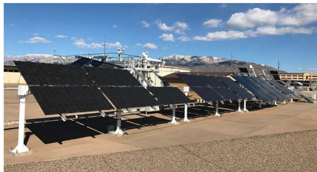
Fig. 1. Two CIGS arrays under test at Sandia
