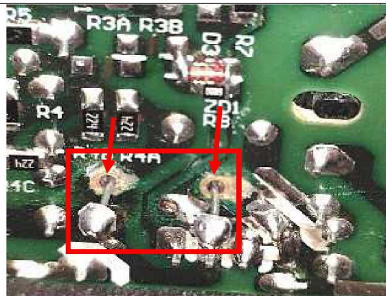
Picture of loose solder structure which holds capacitor in place but is actual very mobile
