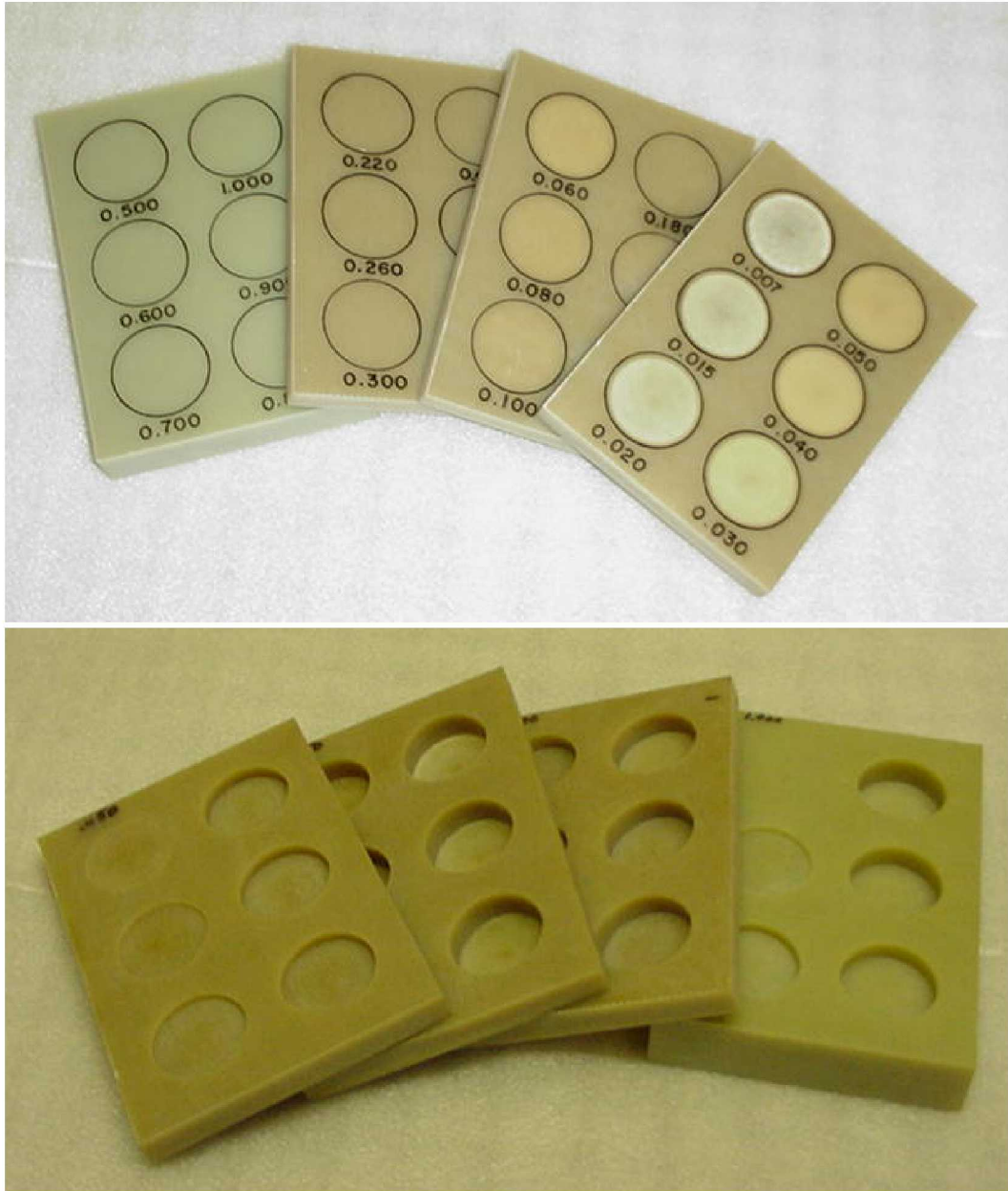
Figure 6-7: Front and Back Photos of G11 Solid Laminate Set with Flat Bottom Holes
