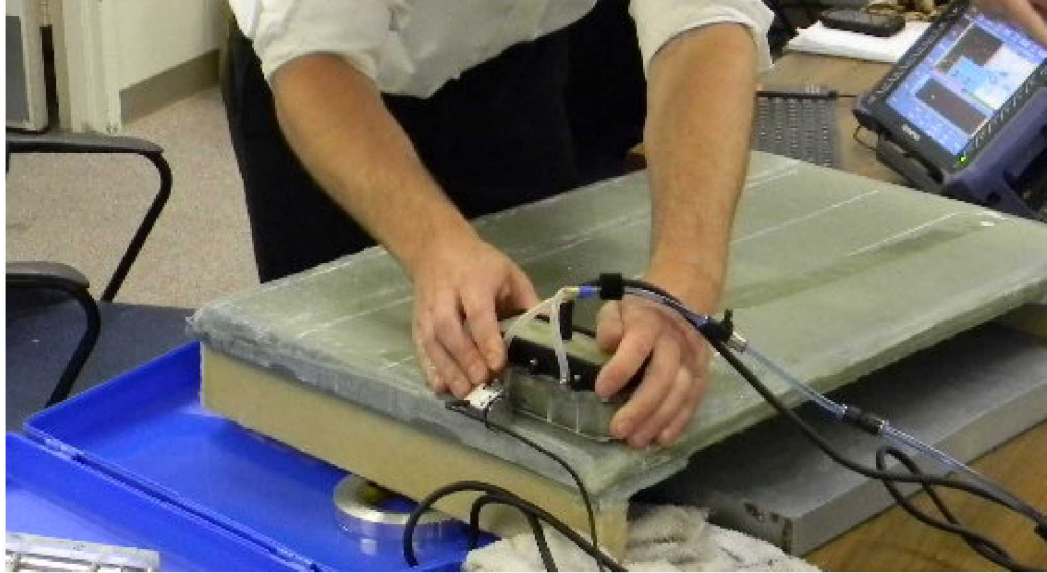
Figure 4-11: Phased Array Ultrasonics Inspection with OmniScan System
