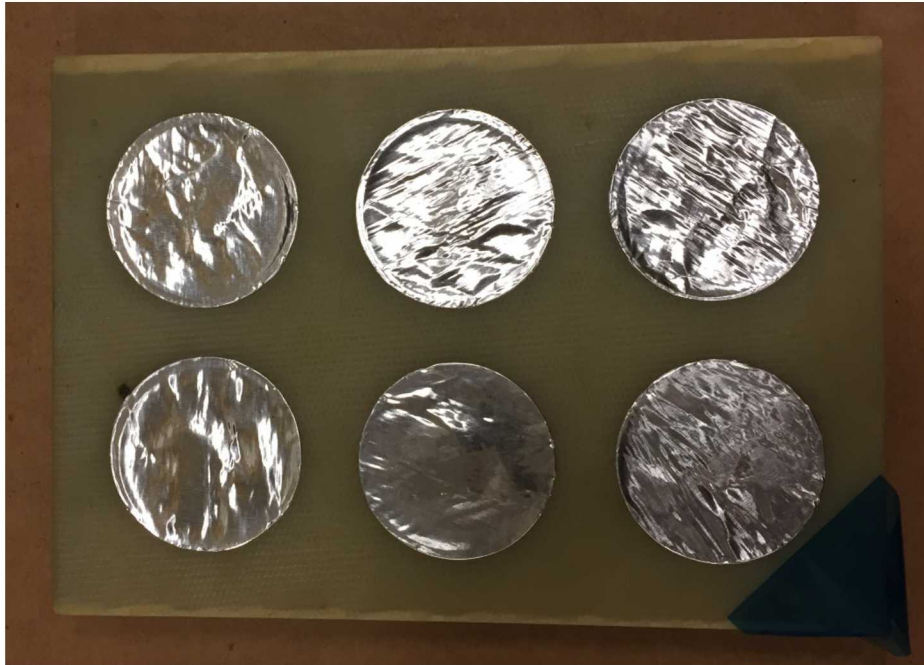
Figure 6-38: Aluminum Tape Added to Rear Surface Over Flat Bottom Holes
