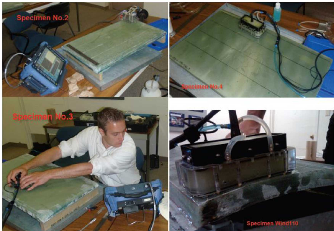
Figure 4-12: Phased Array Probes and OmniScan Deployment on Wind Blade NDI Specimens
