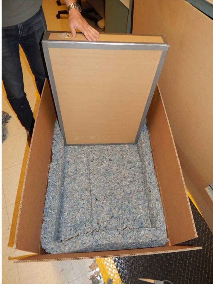
Figure 6-32: Insulated Double Box Construction
