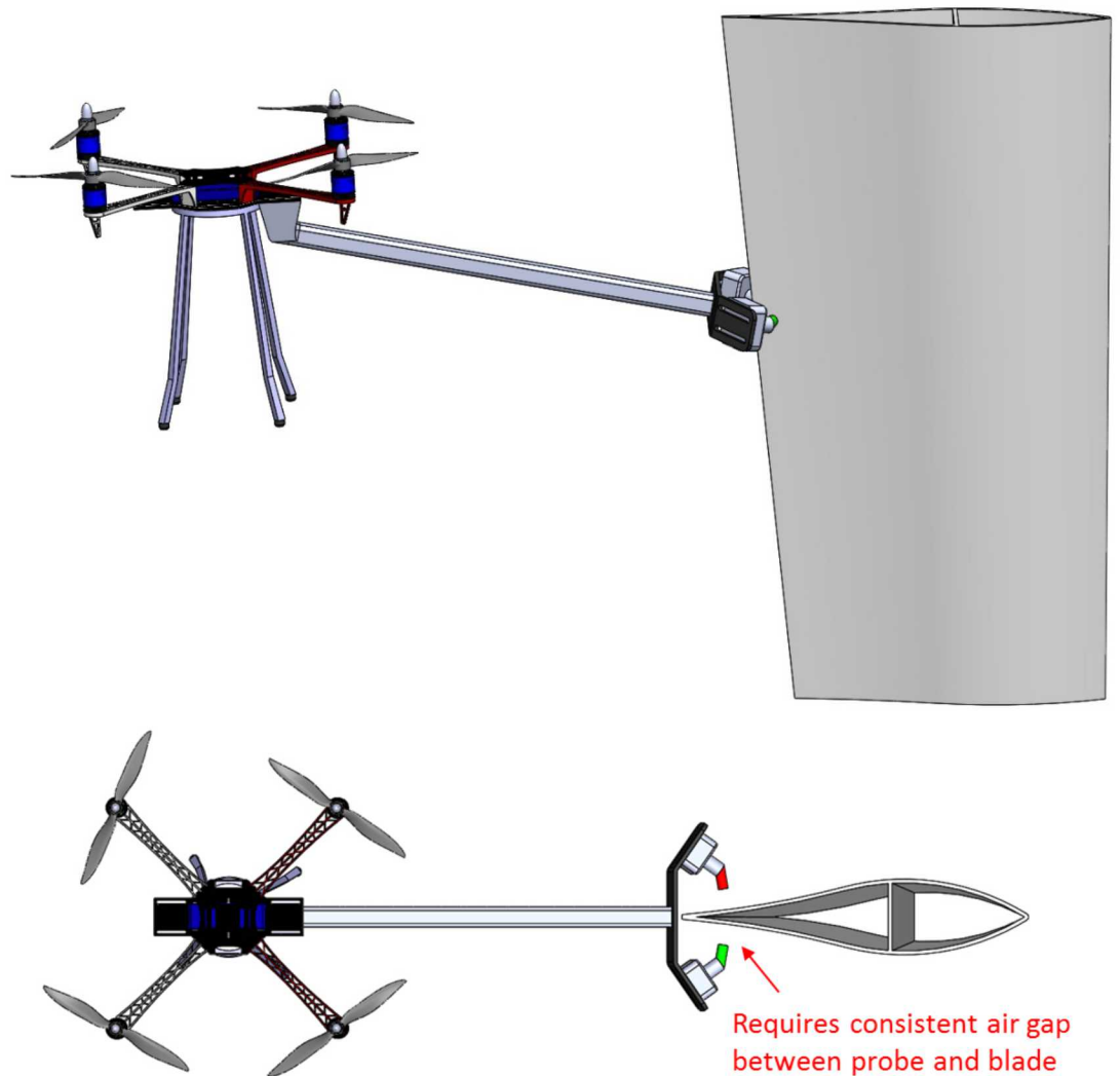
Figure 5-7: Air-Coupled Through Transmission Ultrasonics Drone Integration Concept
