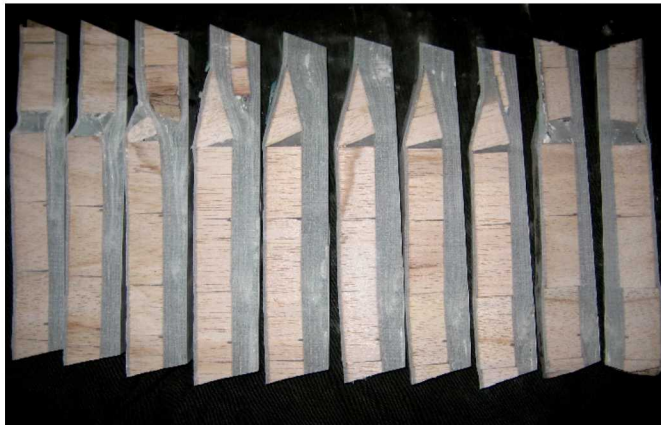
Figure 2-3: “Snowflaking” Flaws in Spar Cap Created by Entrapped Air During Cure
