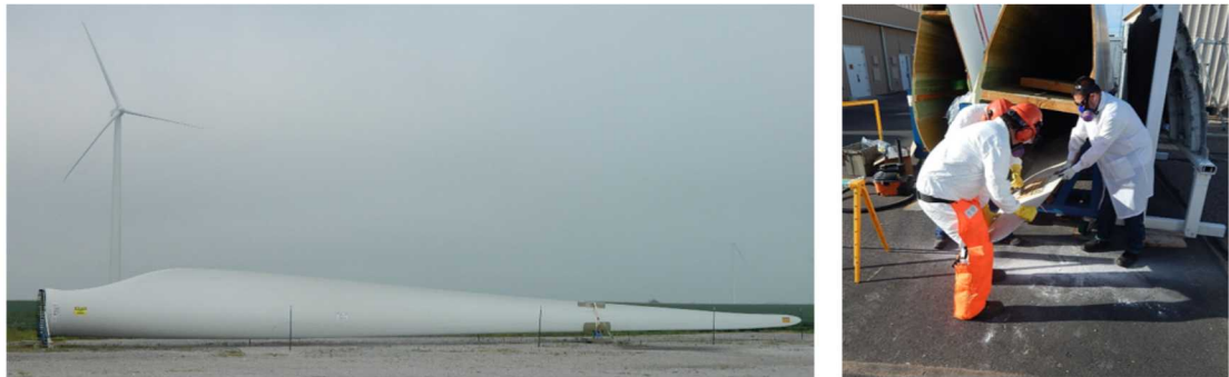
Figure 3-30: Wind Blade Visual Test Specimen FF-V2 Cut From 39m GE Blade, Manufactured by Tecsis
