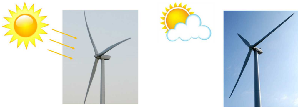
Figure 5-2: Solar Radiation Thermal Gradient Source Concept
