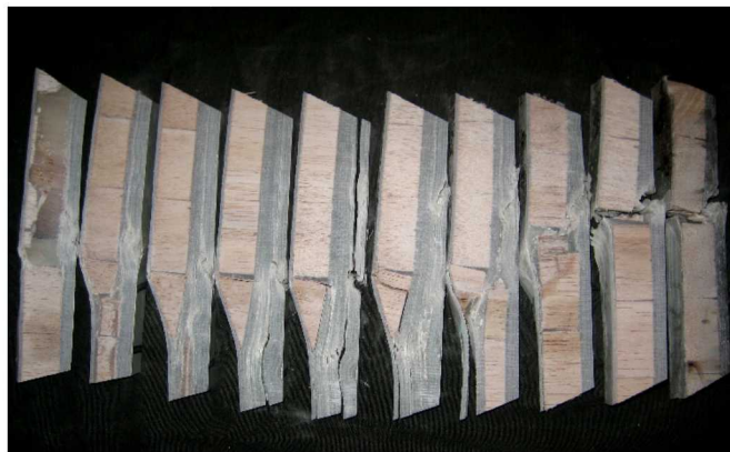
Figure 2-4: Figure Comparing Pristine Blades with Cracks, Delaminations and Other Laminate Fractures that Can Occur in Wind Blades
