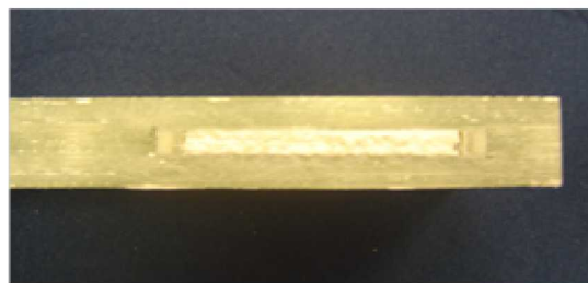
Figure A-20: Cross Section Views of DRY-SPOTS Showing Successful Engineering of Dry Fabric Flaws in Wind Blade NDI Specimens
