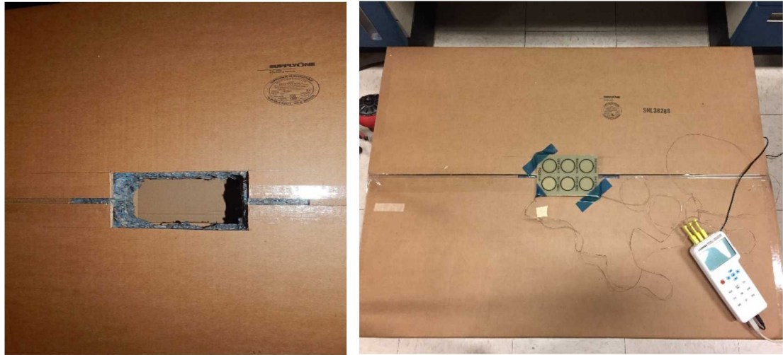
Figure 6-35: Access to Hot Air Cavity to Expose the Rear Surface of the Test Specimens
