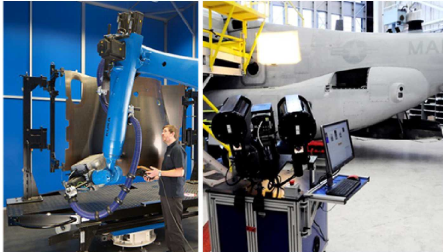
Figure 4-46: Gantry and Projection Thermography Systems for Manufacturing and Large Scale Structural Inspections (images courtesy of Thermal Wave Imaging, Inc.)
