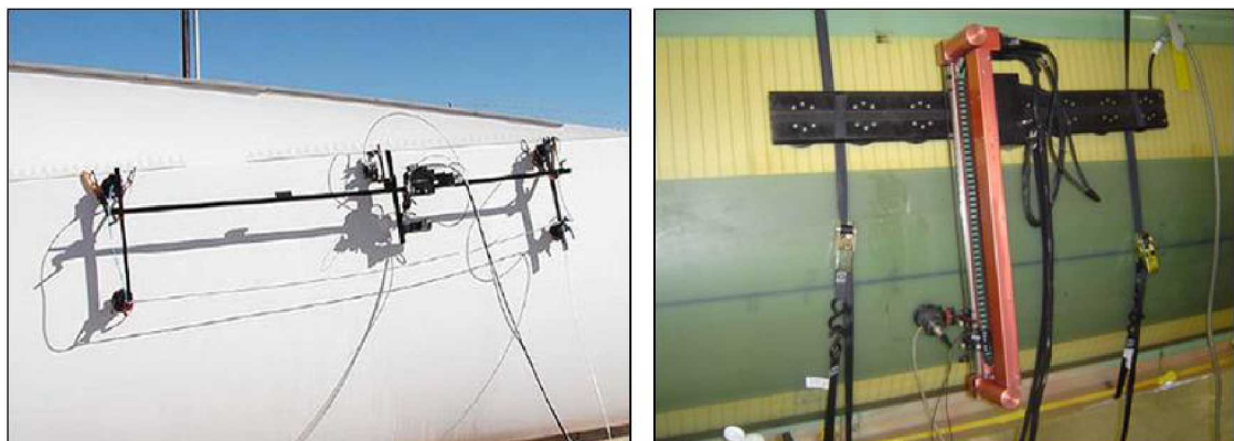
Figure 2-16: X-Y Scanning Systems Can Temporarily Adhere to the Surface of Interest to Produce High-Quality, Through-Thickness Flaw Detection Images Over Wide Areas
