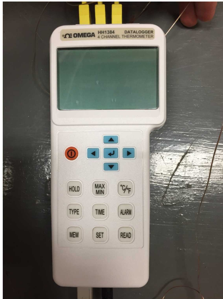
Figure 6-11: Omega HH1384 4-Channel Thermocouple Datalogger with K-Type Thermocouples
