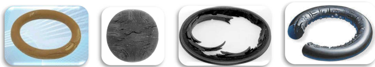
Figure 1. Examples of failures in elastomers in SCO_2 service due to explosive decompression
