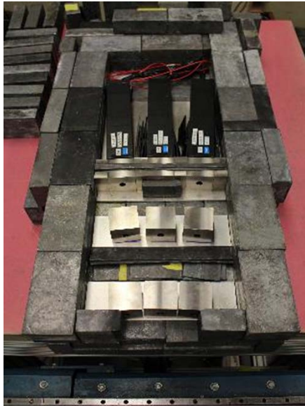
Fig. 7. The three detectors in SPQR are shown with some shielding removed.
