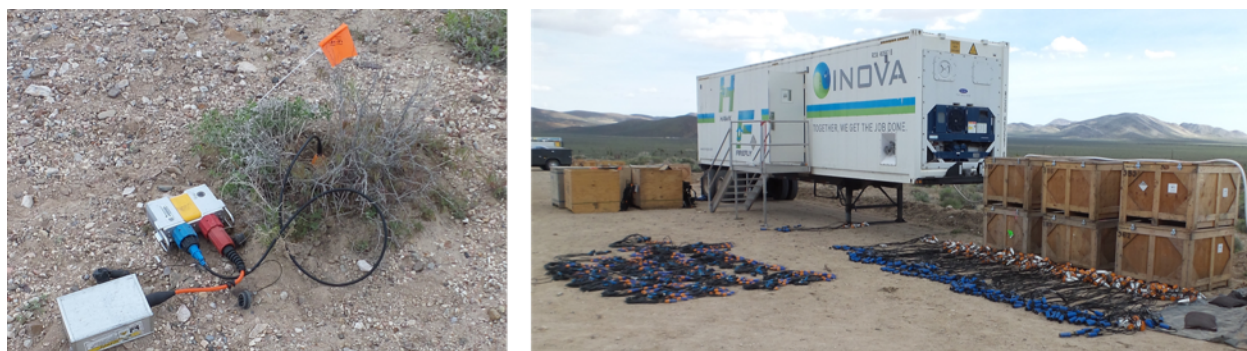
Figure 2. (left) Example of geophone deployment, battery, and digitizer. (right) Truck with field computer and racks for downloading data and charging batteries.
