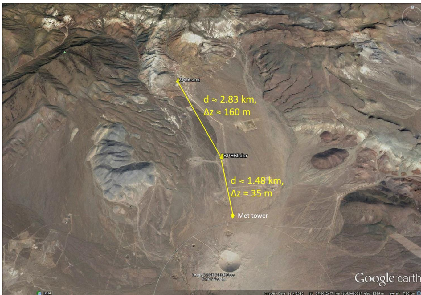
Figure 3: Google Earth image showing the location of the lidar (center) in relation to the SPE6 shot site to the north and NOAA SORD A10AA 10 m tall meteorological tower to the south. The lidar was approximately 2.8 km southeast of the shot and 160 m lower in elevation.
