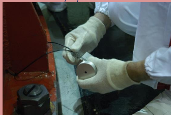
Figure 24. Enhanced fiber optic general purpose seal
