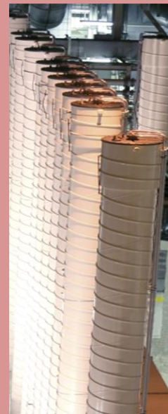
Figure 32. Gas centrifuges operated by the United States Enrichment Corporation are about 45 feet tall and several feet wide
