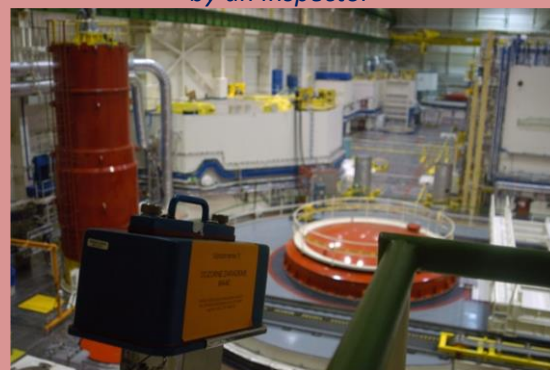
Figure 25. COBRA Seal System being applied by an inspector
