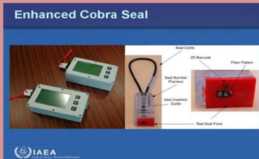
Figure 24. Enhanced fiber optic general purpose seal
