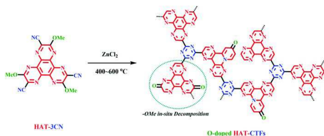
Figure 20. Synthesis route of O-doped HAT-CTFs. Reproduced with permission. [199] Copyright 2015, American Chemical Society.
