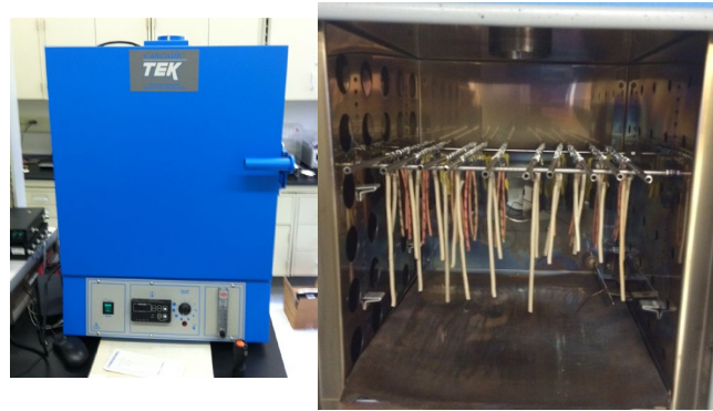
Figure 5. Example of furnace (left) and sample arrangement (right) utilized in accelerated thermal aging of BIW cable insulations.
