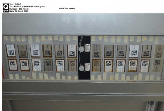
Figure 4: ORNL samples installed in QUV chamber. Samples are shown facing out but were turned inward toward UV lamps for testing.
