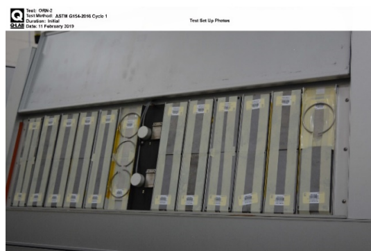
Figure 5: ORNL samples installed in QUV test chamber for UVA testing.
