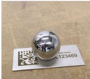
Figure 9: Impact testing allowed a 500 g smooth steel sphere to fall from 1000 mm onto each of the samples.
