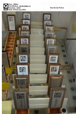
Figure 6: ORNL samples installed in Q-Fog test chamber.
