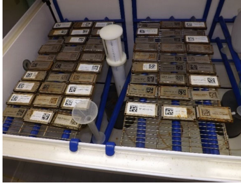
Figure 8: ORNL samples installed in salt fog chamber
