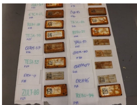
Figure 10: Image of selected samples after cyclic corrosion testing.
