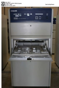
Figure 3: ORNL samples installed in Q-SUN Xe-3 Xenon arc test chamber.
