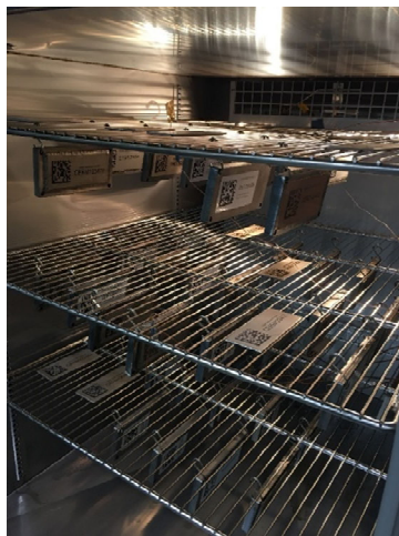
Figure 7: ORNL samples in Tenney TC20RC environmental enclosure.
