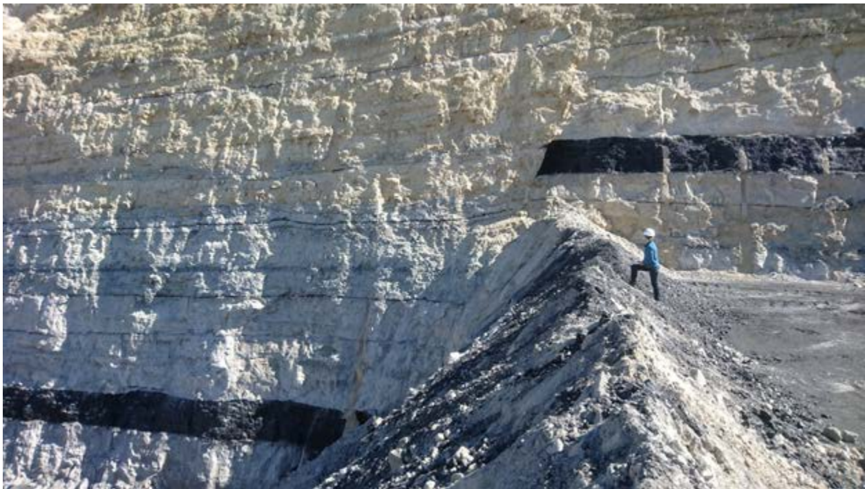
Figure 4.2.2. Normal faulting, highlighted by offsets in a coal seam, east of the JBP at the Bridger mine high wall.
