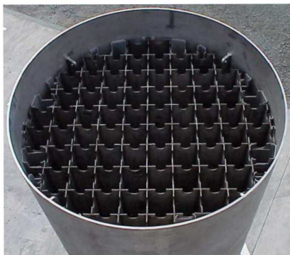
Top view of MPC-68 shell and basket (Greene et al. 2013).
