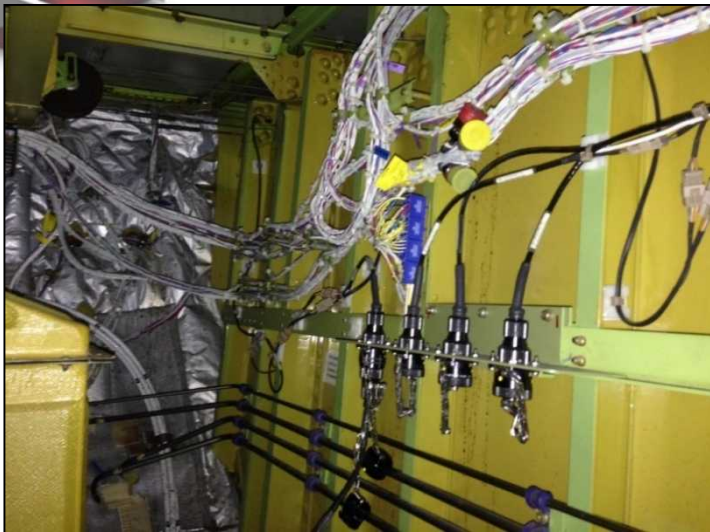
Connecting SLS Leads and Running PM-200 to Monitoring Device to Check Sensor Network
