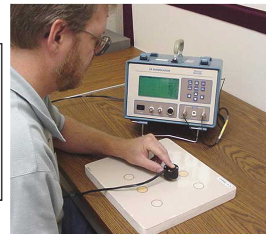
Corrosion Detection with Dual Frequency Eddy Current
