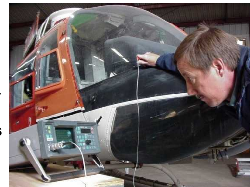
Corrosion Detection with Dual Frequency Eddy Current
