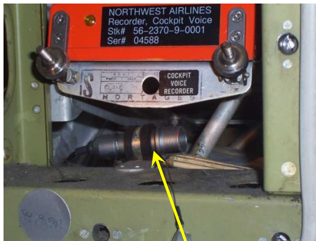
SLS connector routed to access panel
