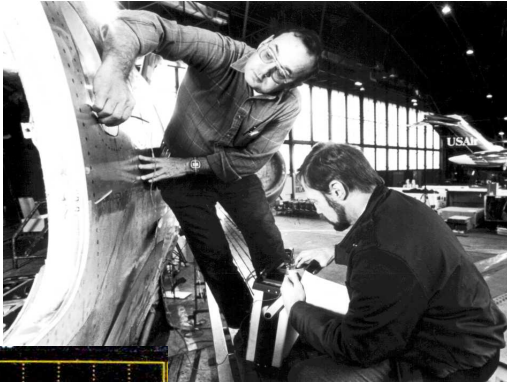
Eddy Current Signal at Crack Site
