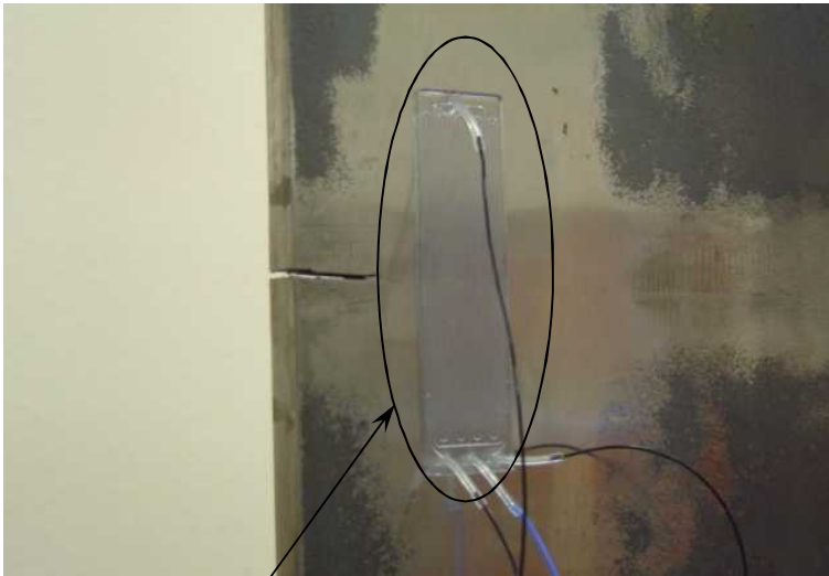
CVM Sensor Adjacent to Crack Initiation Site
