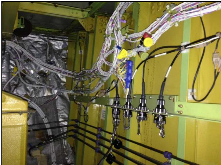
Running PM-200 Monitoring Device to Measure dCVM Levels of Each Sensor Group
