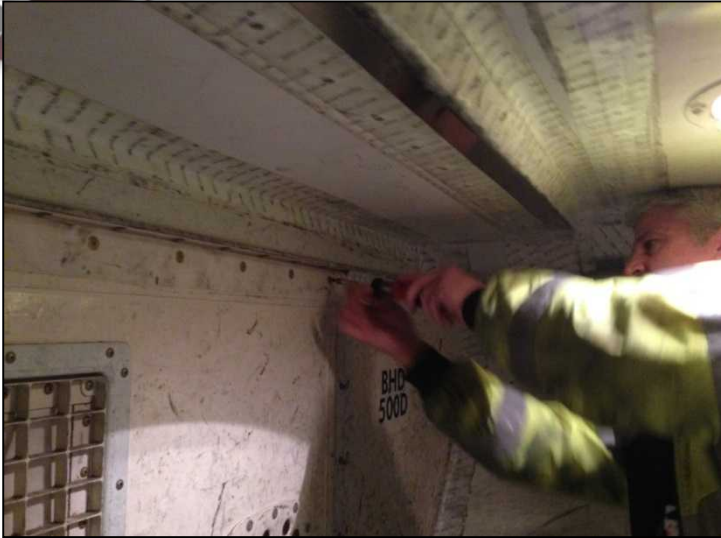
Reinstallation of Forward Baggage Liner and Close-Up of Compartment
