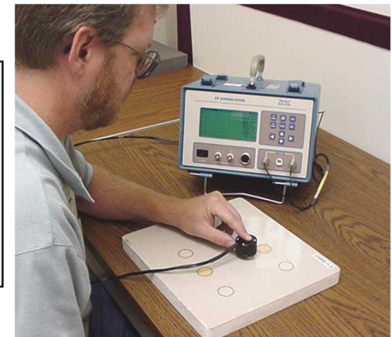
Corrosion Detection with Dual Frequency Eddy Current
