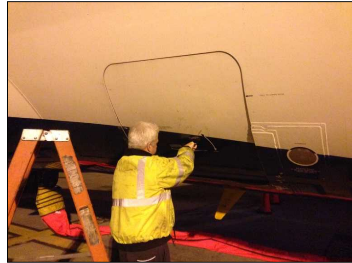
Reinstallation of Forward Baggage Liner and Close-Up of Compartment
