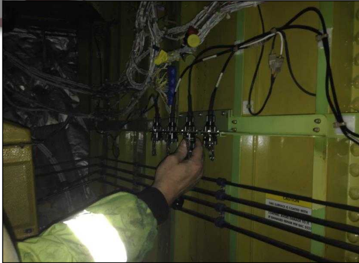
Connecting SLS Leads from PM-200 to On-Board SLS Connectors
