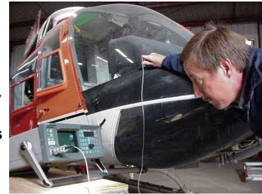
Corrosion Detection with Dual Frequency Eddy Current
