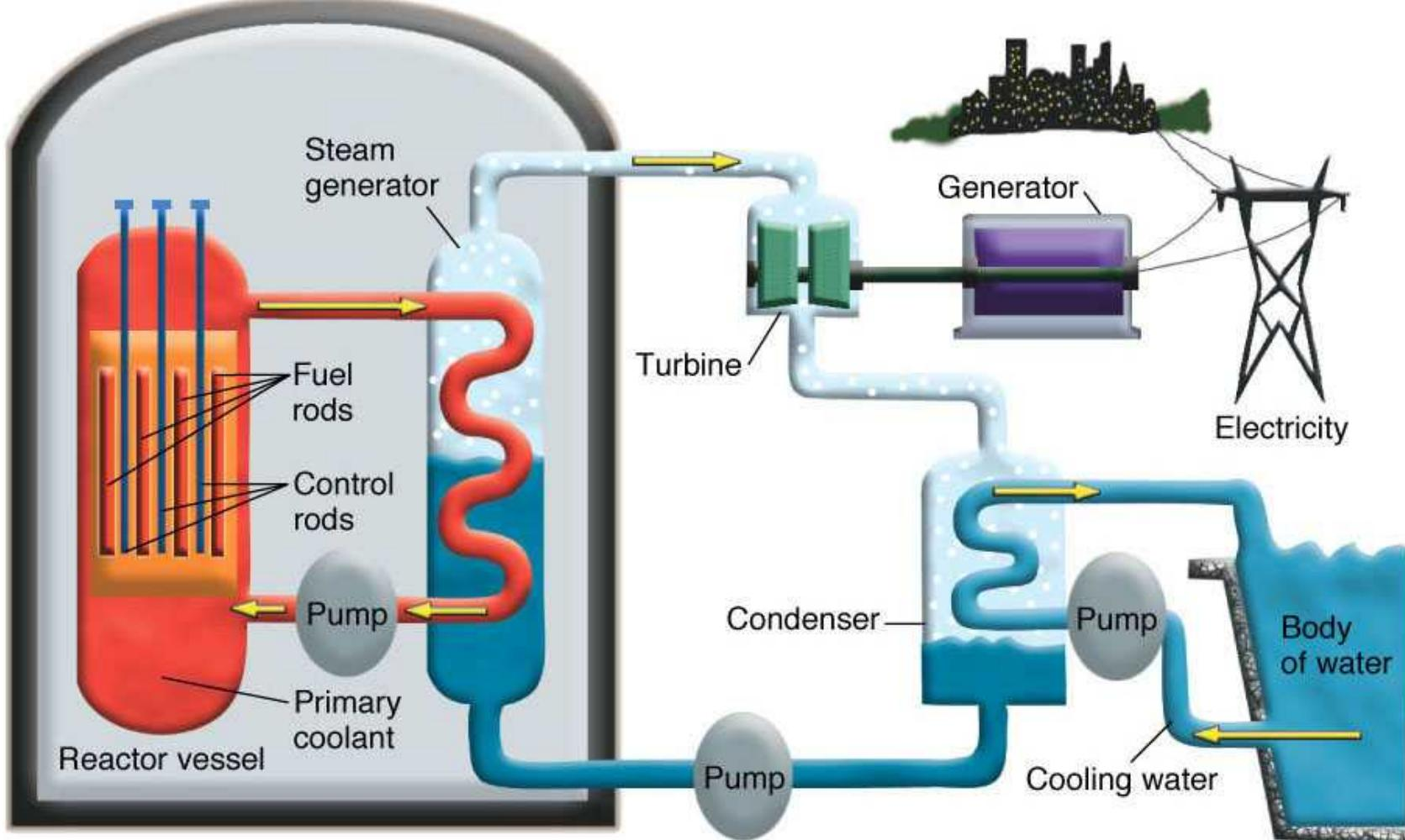
A nuclear reactor, shown here schematically, produces heat that converts water to steam. The steam powers a turbine, just as in a conventional coal-burning plant.
