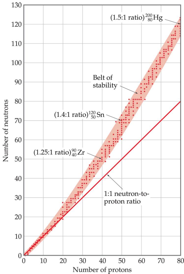
More protons require more neutrons to provide a compensating nuclear strong force and to dilute the electrostatic proton-proton repulsions. The plot stops at element 83 (bismuth) because no element above this has a *stable* isotope.
