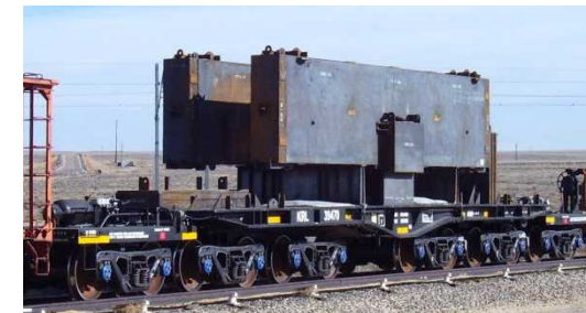
PFS 2043 rail car with mass loading @ TTCI
