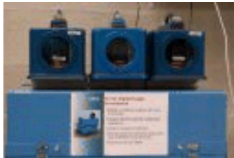
Cameras in their secure housings used for remote monitoring of nuclear sites. Source: IAEA/Dean Calma
