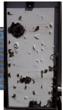
Delamination in a solar cell
