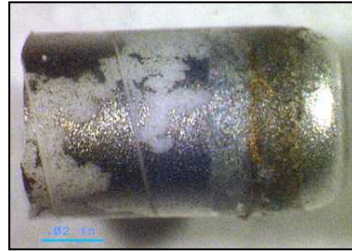
NiCr Resistor Corrosion
