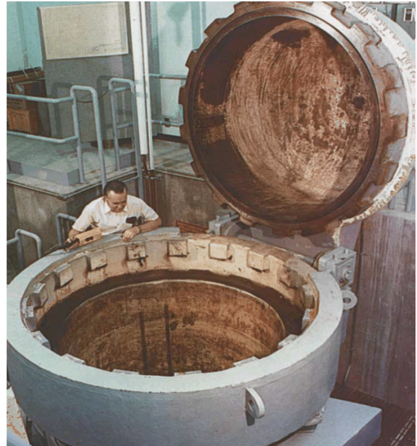
Hydrostatic testing vessel, AECL/Whiteshell
