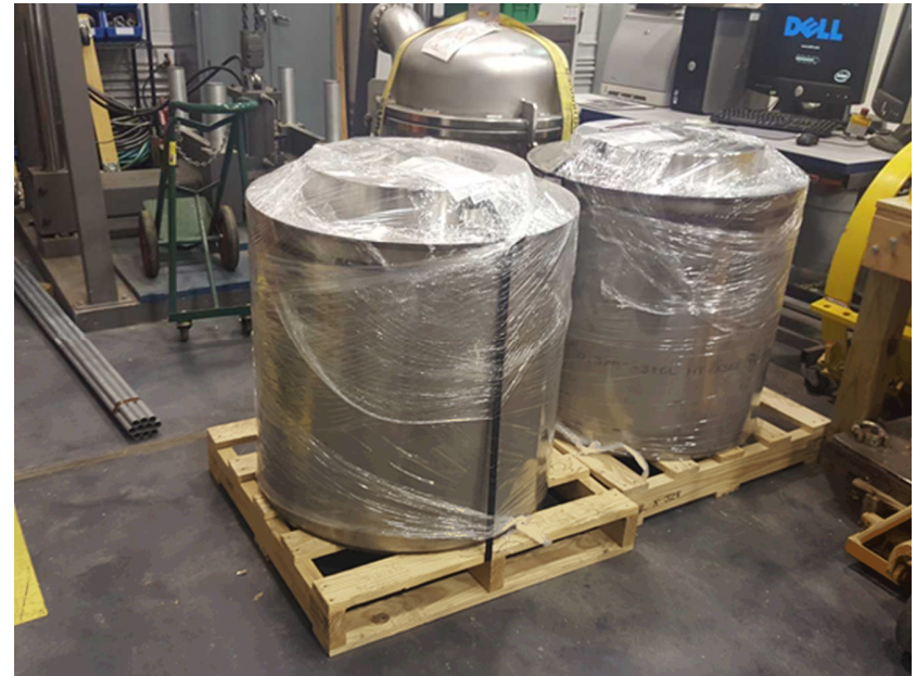
Weld-test mock-ups from ORNL standardized canister test program.
