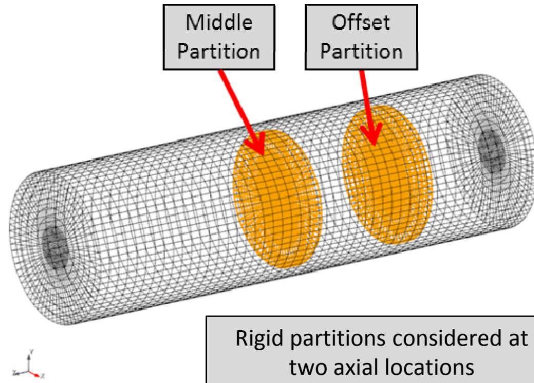
Disrupt the acoustic mode shape by adding a partition
