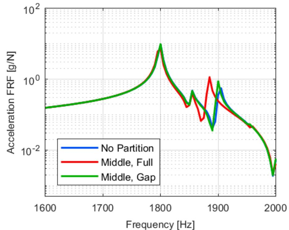
Disrupt the acoustic mode shape by adding a partition
