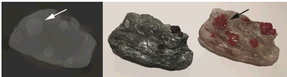
Figure 6 - Alaskan Almandine garnet; slice from scan (left), rock (center) and 3d print (right). Arrow indicates internal crystal visible only in scan and 3d print.
