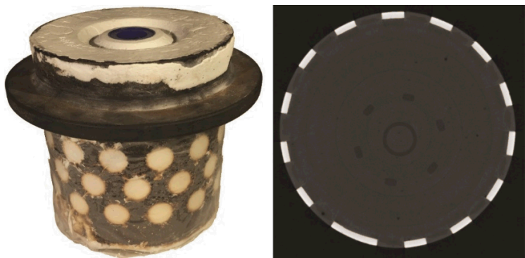
Figure 15 - Casting flask (left) and x-ray CT slice (right).
