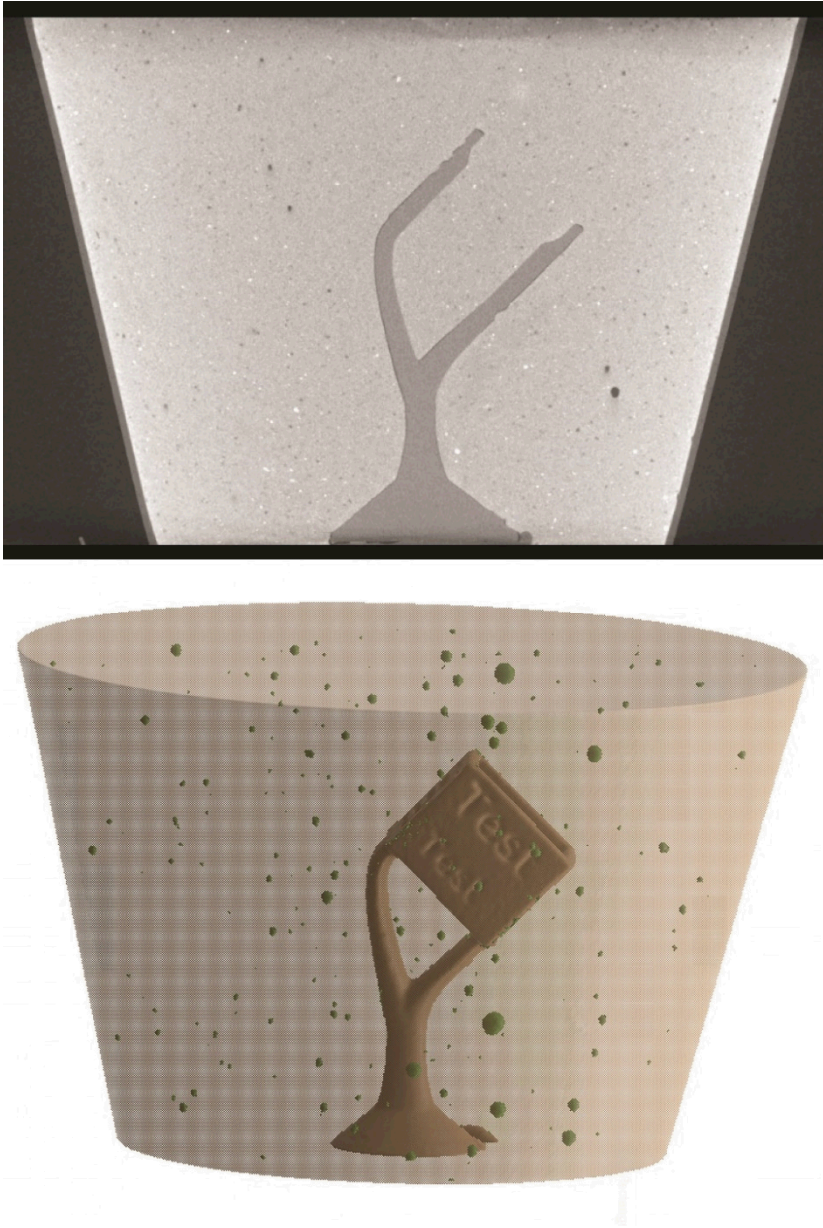
Figure 18 - Results from the CT of sample #3. A slice through the reconstructed volume (right) and the processed volume segmented into each material (wax, voids, and plaster) (left).
