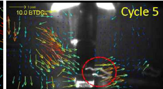
Simultaneous flow & spark channel imaging (M. Sjöberg) (OEM)
