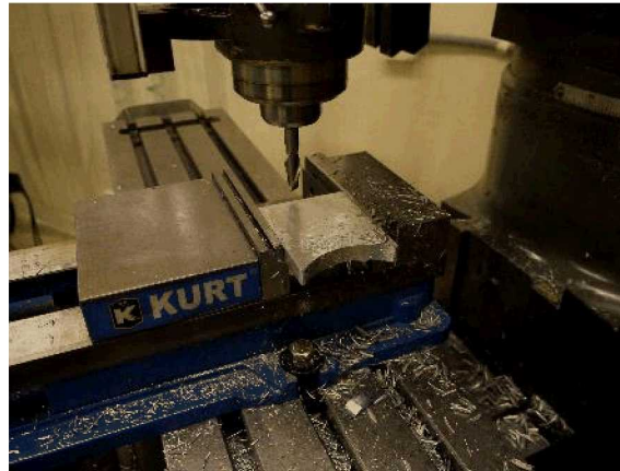
Milling machine with part mounted in vise for machining. Above is an end mill cutter that will machine the aluminum.
