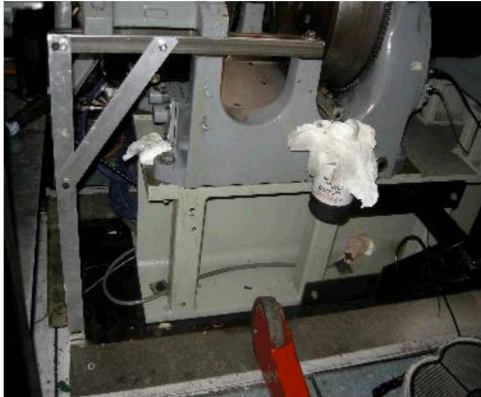
Engine modification: fabrication of temporary support stand on left.
