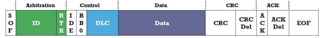
Fig. 1: Image from Cho & Shin [18] of CAN 2.0 data frame. 11 bit arbitration ID field used for prioritization of messages. Up-to eight byte data field used for message contents.
