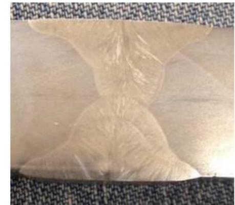
Weld zone, 304 SS plate. Photo: Ranor
