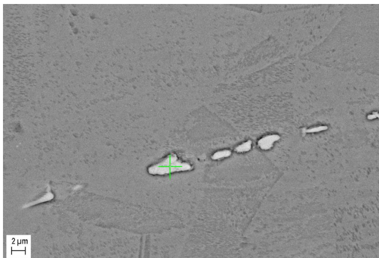
Figure 6.3. SEM SE image showing Nb rich MX precipitates found in the as-received Alloy 709.
