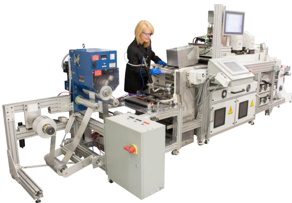
Figure 9. Miltec roll to roll, slot die coater and 3 UV lamp laboratory system
